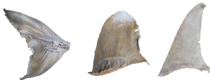
The replica shark fins after 3D printing, using sintered nylon as printing compound (as seen from left to right: Bowmouth Guitarfish caudal fin, Oceanic Whitetip Shark dorsal fin, and Great Hammerhead Shark dorsal fin)
