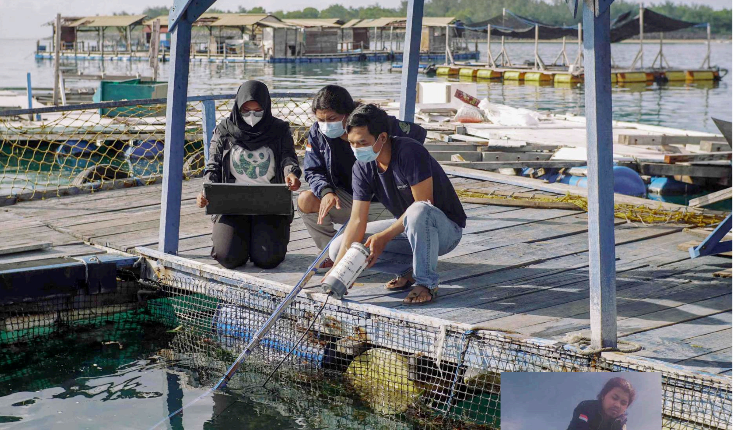
Lab-scale trial of the new ESS conducted in the Serangan floating net cage with sharks. These trials were conducted to find the most optimal current strength or frequency setting to deter the sharks. © WWF-Indonesia / Novi Anastasya
